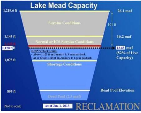
Figure 7 Lake Mead IOPP Schematic
