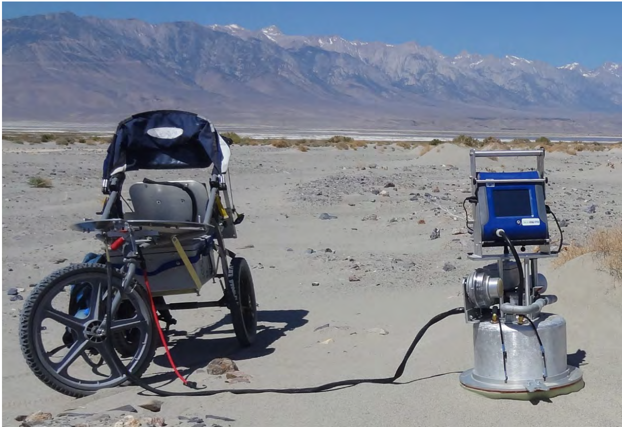
Figure 1. PI-SWERL Unit and Carrier
