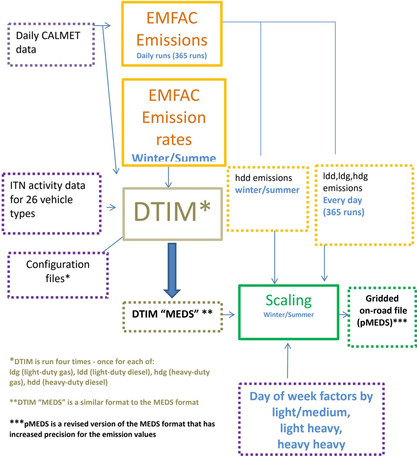
Figure 3 Block diagram for on-road processing
