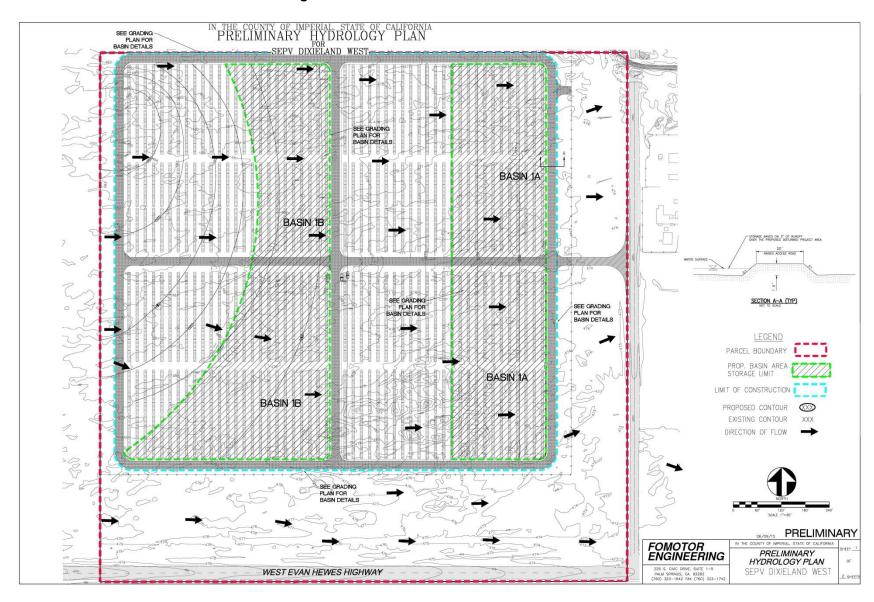
Figure 4.9-3. Direction of Water Flow on DWSF
