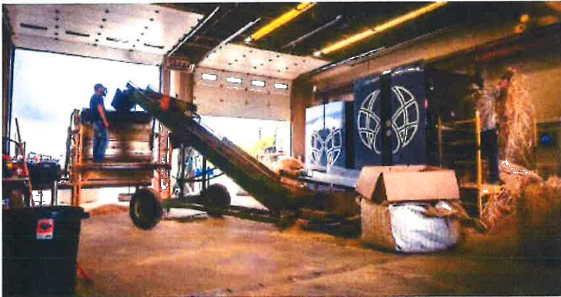
Sample decorticated equipment been fed hemp stalk and outputting processed material.
