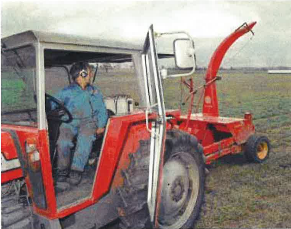
Figure 8 Tractor PTO-powered trailed forage harvester with mechanical controls
