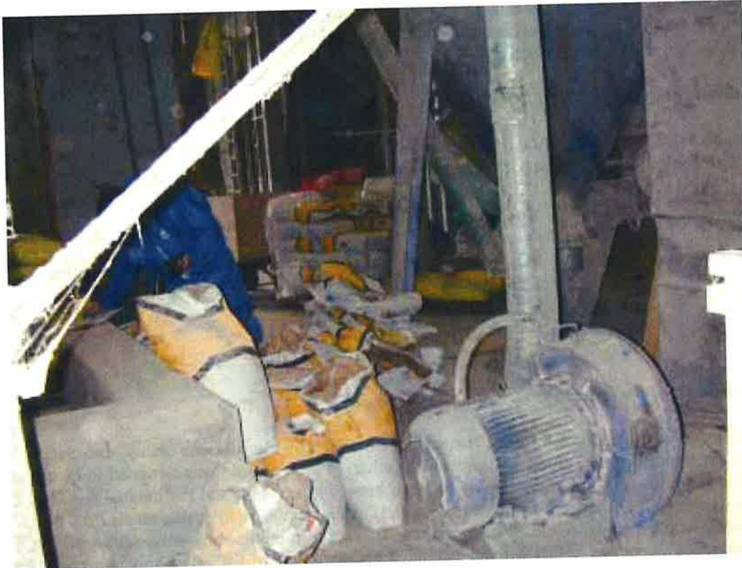
Figure 15 General view of animal feed preparation building with hammer mill shown in the foreground
