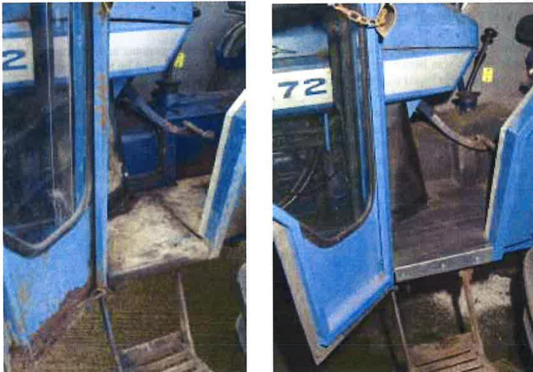
Figure 26 Dilapidated (left) and refurbished (right) tractor Q-cab
