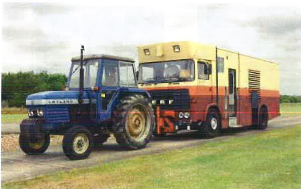
Figure 25 Measurement of test tractor in-cab noise level during drawbar loading
