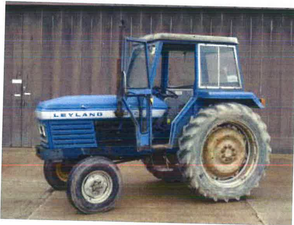
Figure 10 Deteriorated Q-cab on otherwise serviceable 70hp tractor
