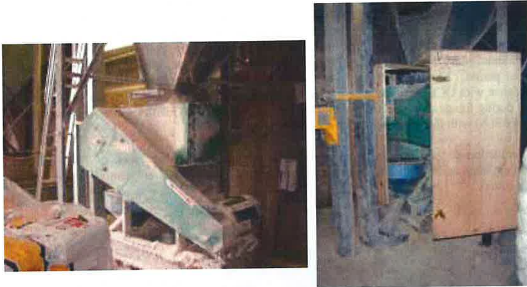
Figure 17 Animal feed cubing machine installation, before (left) and after (right) noise reduction treatment (noise reduction enclosure shown open for machine maintenance)
