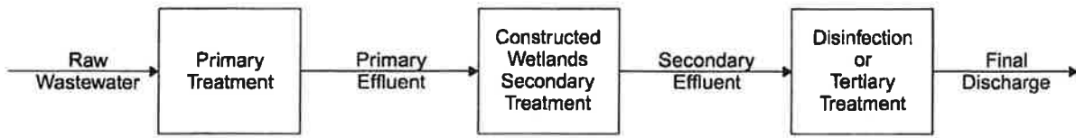
Figure 2-1. Constructed wetlands in wastewater treatment train
