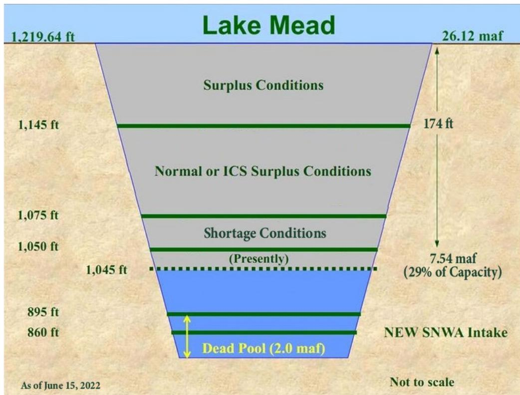
Figure 7. Lake Mead Schematic (June 15, 2022)
