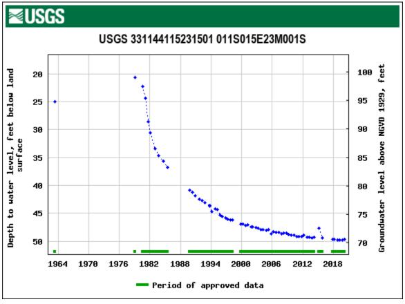
FIGURE 5. USGS Groundwater Level Hydrograph
