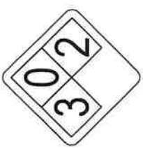
ALERTING SIGN (FOR CELL SITE BATTERIES)
