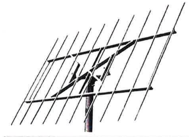
Typical dual axis mounting structure
