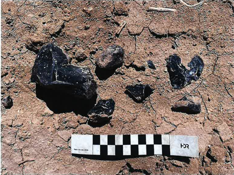
Figure 8. obsidian nodules and fractured pieces observed on the embankment and embedded in the road surface
