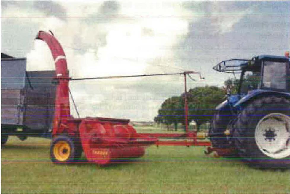
**Figure 19** Tractor (with rear window open), trailed forage harvester and trailer
