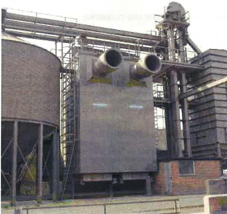
**Figure 7** Large, continuous-flow grain drying installation
