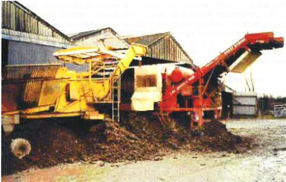
**Figure 5** Sugar beet cleaner/loaders with manned pick-off platforms
