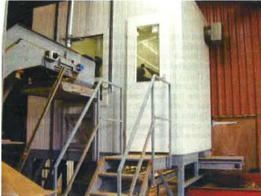
**Figure 22** Dedicated operator station on onion grading line
