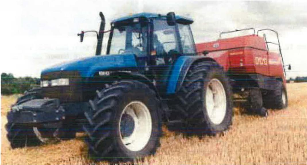
**Figure 18** High density baler typical of PTO driven implements
