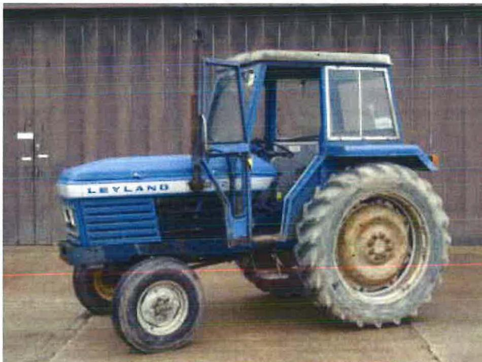
**Figure 10** Deteriorated Q-cab on otherwise serviceable 70hp tractor
