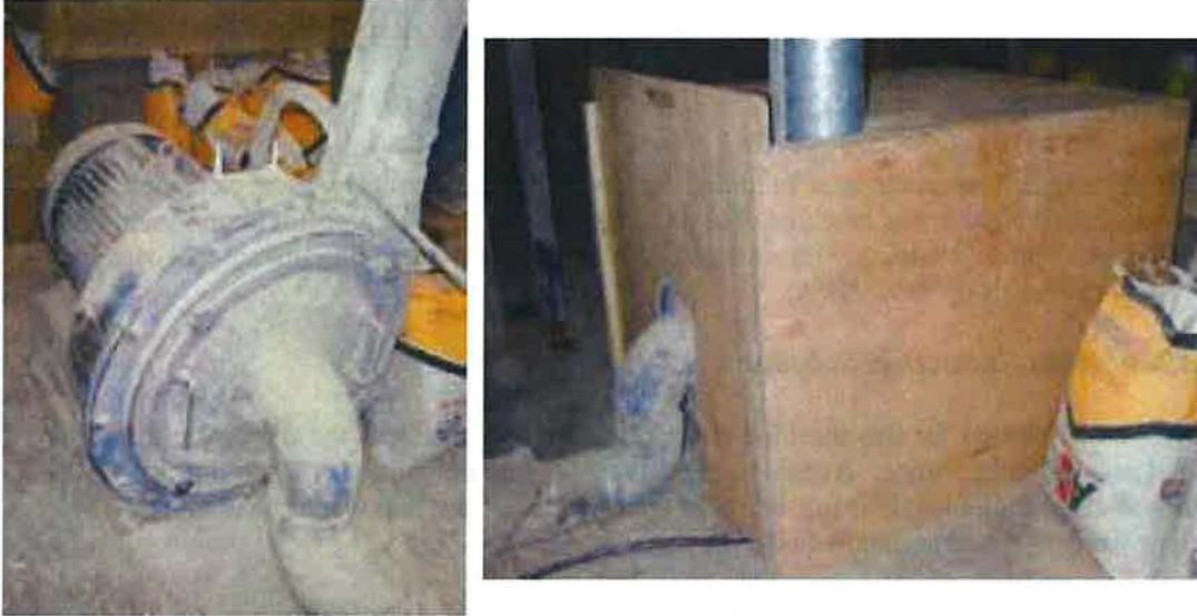
**Figure 16** Hammer mill installation, before (left) and after (right) noise reduction treatment
