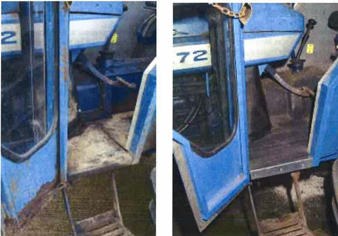
**Figure 26** Dilapidated (left) and refurbished (right) tractor Q-cab
