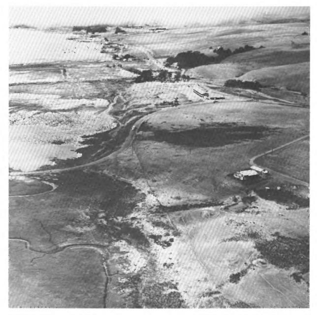
FIGURE 2.9. – A scarp facing the Pacific Ocean, with marine terraces above, marks trace of the San Andreas fault at Bodega Bay, 70 km north of San Francisco. View northwestward.
