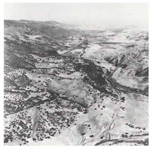
FIGURE 2.15.—The San Andreas fault about 40 km south of San Juan Bautista. Here, the Calaveras and San Andreas faults join. The Gabilan Range is on left; the San Benito River meanders across fault zone. View northwestward.
