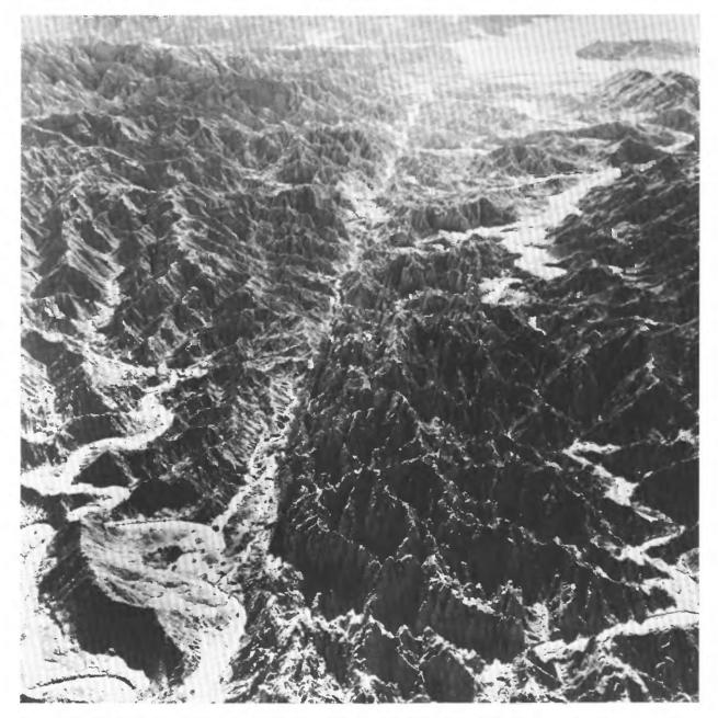
FIGURE 2.33.—The San Andreas fault in badlands of the Mecca Hills, Coachella Valley. Sympathetic slip of as much as 1+ cm occurred here during the Borrego Mountain and Imperial Valley earthquakes of 1968 and 1979, respectively.
