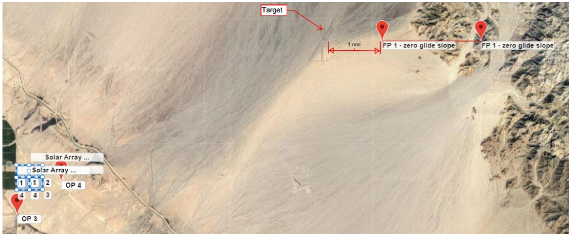
Figure 1: Wister Solar Project PV Array Layout in ForgeSolar depicting FP as requested by the USMC
