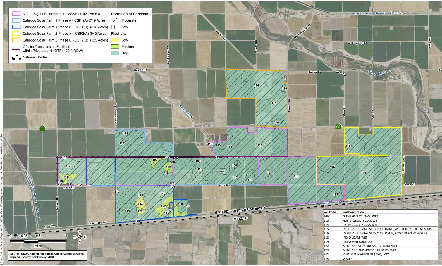
These clayey materials are generally comprised within one or more soil horizons within the upper five feet of the soil profile. Similarly, corrosive soils can damage underground utilities including pipelines and cables, and can weaken roadway structures. Soils within project study areas are classified as moderately corrosive to concrete and steel (see Figure 4.6-2) (NRCS 2008). These hazards are discussed further in the impact analysis.
